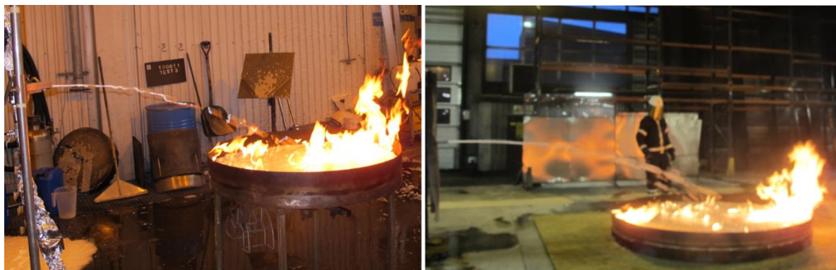
Figure 13. SP Method 2580 (left) is a down-scale of the larger test according to the European standard EN 1568-3 (right).
