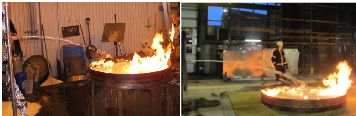
Figure 12. SP Method 2580 (left) is a down-scale of the larger test according to the European standard EN 1568-3 (right).
